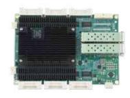
EPS-24G4X-HSP EPS-24G4X Managed 28-Port Gigabit Ethernet Switch with 4 10G SFP+ Ports Test Standard: MIL-STD-202H
